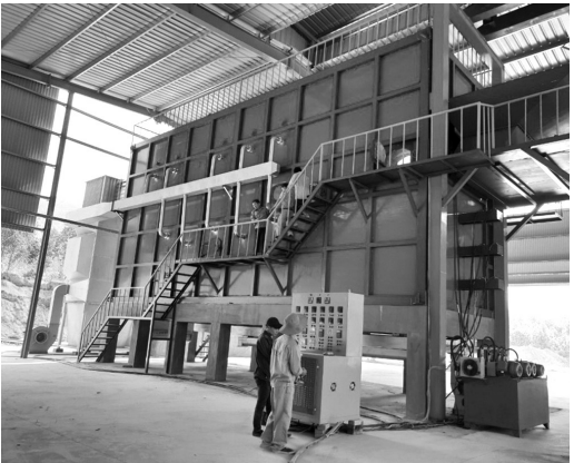
▲ Domestic waste incinerators with a capacity of treating 50 tons of waste/day of the T - Tech Nghệ An Joint Stock Company
