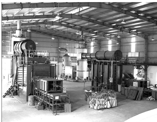
▲ Industrial waste incinerators with a capacity of 1,000 kg/h of the Green Industrial Environment Company Limited in Vĩnh Phúc are supported with loans by the Fund
